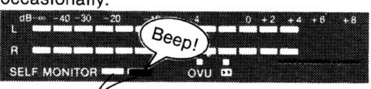
The recording is not good when both the white and red indicators blink. An alarm will sound when the red indicator blinks. Check that the head is not contaminated or that the recording level setting is not too high.
